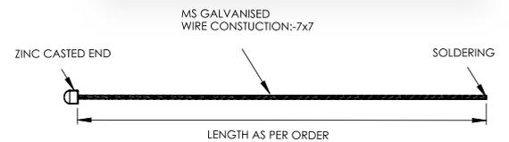
**Cable:** After selecting the Channel, the next step is to choose the hanging option, which can be Cable.
